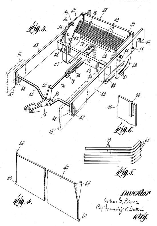
ALIGNING DEVICE FOR MANIFOLDING TYPEWRITERS
