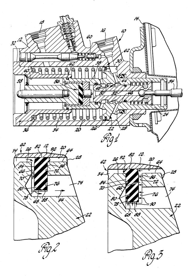
HYDRAULIC MOTOR SEAL AND VALVE
