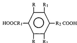
wherein R, R<sub>1</sub>, and R<sub>2</sub> are as defined herein. The ring between the two chains can either be a 6 membered ring as shown, or a 5 membered ring; and there are generally 6 to 12 carbon atoms between the two carboxyl groups. The total number of carbon atoms is generally about 36.
