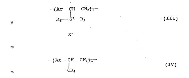
wherein R₄ and R₅, which may be the same or different, each represents an alkyl group, R₅ represents a lower alkyl group, X represents a halogen atom or a halogen compound, Ar represents a p-phenylene group, a 1,4-naphthylene group, a 2,5-thienylene group, or a 2,5-furylene group, each of which groups may have a substituent group, and n represents an integer of 8 or more.
