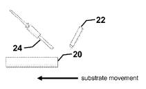
(57) Abstract: A method for cleaning a substrate having organic and inorganic residues disposed thereon is provided. The method includes removing organic residue from the substrate using atmospheric oxygen plasma, and removing inorganic residue from the substrate using cryogenic C02. The substrate may be pretreated using a benign cooling agent, and post-treated using a dilute wet chemical cleaning method.
