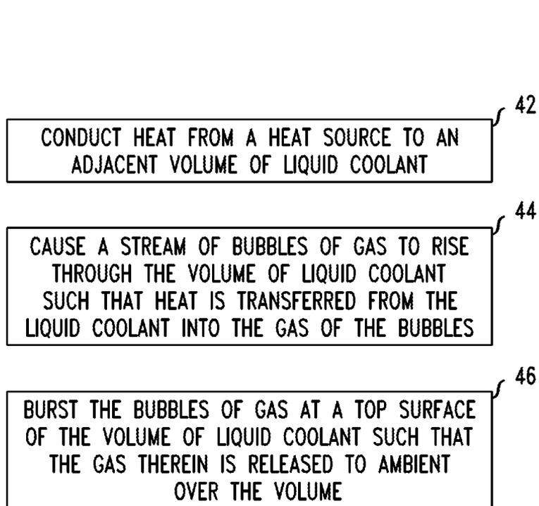
**COOLING WITH LIQUID COOLANT AND BUBBLE HEAT REMOVAL**
