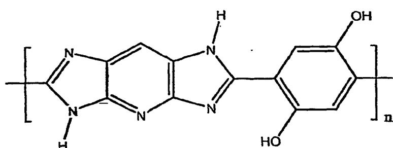
[0038] Polypyridobisimidazole fiber can be distinguished from the well known commercially available PBI fiber or polybenzimidazole fiber in that that polybenzimidazole fiber is a polybibenzimidazole. Polybibenzimidazole fiber is not a rigid rod polymer and has low fiber strength and low tensile modulus when compared to polypyridobisimidazoles.
