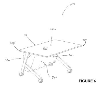
(57) Abstract: The present invention may be said to consist in a desk arrangement which is capable opening up to receive computer and peripheral equipment for storage and transport. The desk arrangement is also configured for storage in a compact formation, and preferably nested together with similar desk arrangements.
