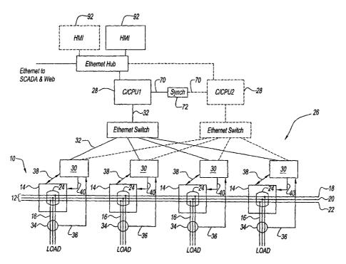
(57) Abstract: A circuit breaker lockout device (26) is provided that prevents the breaker contacts from being closed when the circuit breaker (14) is in a lockout state in response to a lockout signal and permits the breaker contacts to be closed when the circuit breaker is in an enabled state in response to an enable signal.
