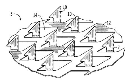
(57) Abstract: An apparatus for transdermally delivering a biologically active agent to a patient comprising a microprojection member (5) having a plurality of microprojections (10) that are adapted to pierce the stratum corneum of the patient, the microprojection member having a biocompatible coating (16) disposed thereon that includes a biologically active agent selected from the group consisting of peptide and protein conjugates.
