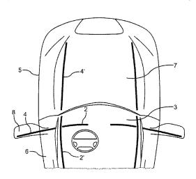
created by the second section (4, 4') of the illuminating fixture is radiated such that it is visible from a definable position relative to and outside of the vehicle (1).
