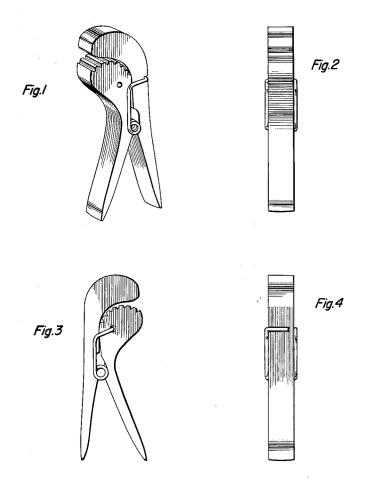
FIG. 1 is a perspective view of a clothespin showing my new design;
