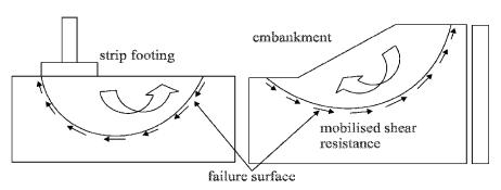
At failure, shear stress along the failure surface reaches the shear strenght.
