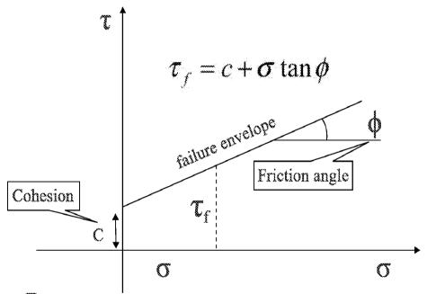
If is the maximum shear stress the soil can take without failure, under normal stress of  $\sigma$ .
