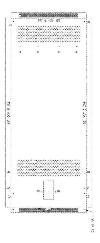
HOLE A: 4 PLACES, 0.26" DIA HOLE B: 8 PLACES, CS FOR 8-32 FLATHEAD SCREW, ON OUTSIDE SURFACE HOLE C: 2 PLACES, 0.18" DIA
