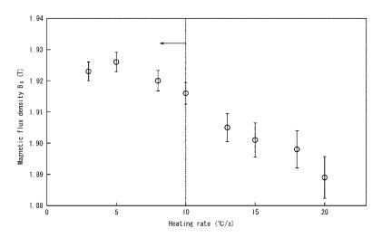
in final intermediate annealing, heating is performed at a heating rate of  $10^{\circ}$  C./s or less for 10 sec or more and 120 sec or less in a temperature range of  $700^{\circ}$  C. or more and  $950^{\circ}$  C. or less.
