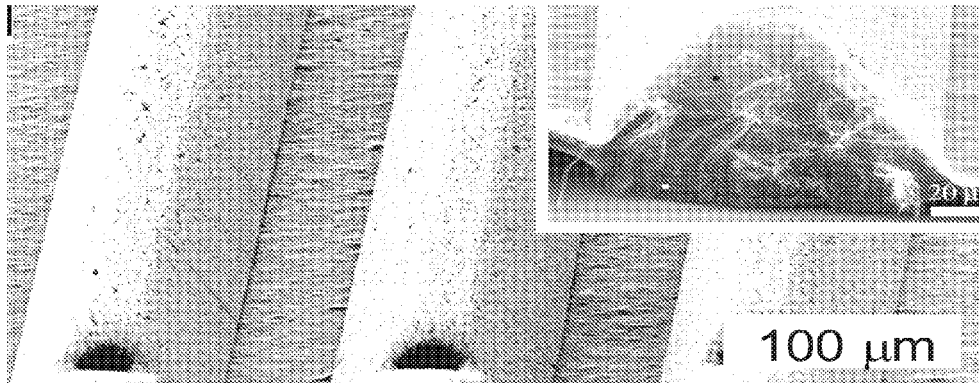
PRIOR ART "Grow-Molded" CNT Microstructures
