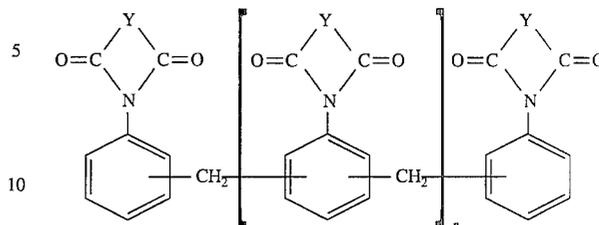
in which Y is a substituted or unsubstituted divalent radical having at least 2 carbon atoms, preferably 2 to 6 carbon atoms, and a carbon-carbon double bond and n is a number having an average value of 0 or greater, preferably an average value from about 0 to about 4. Such polymaleimides are disclosed in U.S. Pat. No. 4,298,720, for example. Specific examples of such compounds include polymethyl-enephenylenemaleimides having the formula
