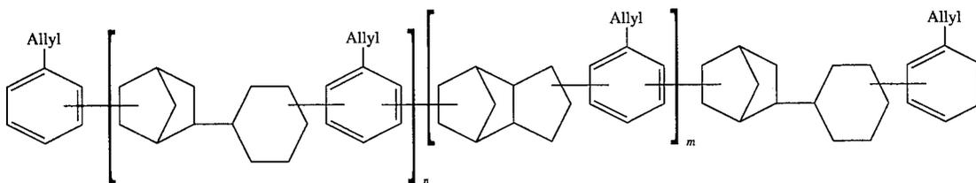
in which Allyl is an allylic ether group and each of m and n is a number within the range of 0 to about 10. The phenolic allyl ether compounds are useful with polymaleimide as the resinous component of electrical laminating and encapsulation formulations.
