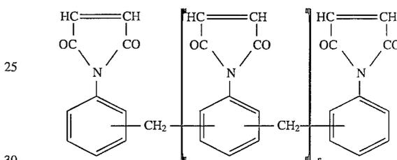
in which n is a number having an average value of 0 or greater, preferably an average value from about 0 to about 4. These polymaleimides can be obtained by reacting an aniline-formaldehyde condensation product with maleic anhydride as described in the above patent.
