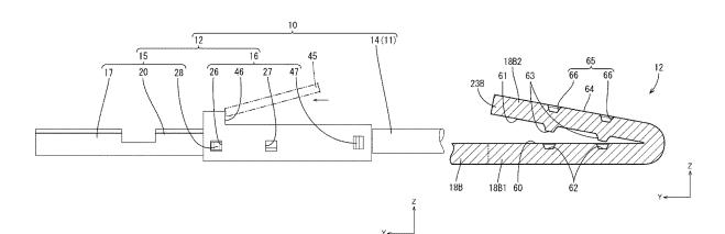
the overlapping portion and a second facing surface of the tip portion are facing each other and overlapped.
