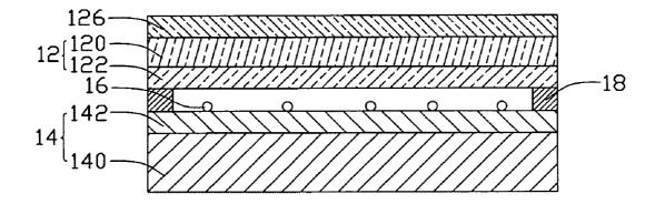
providing at least one array of carbon nanotubes, a first substrate, and a second substrate
