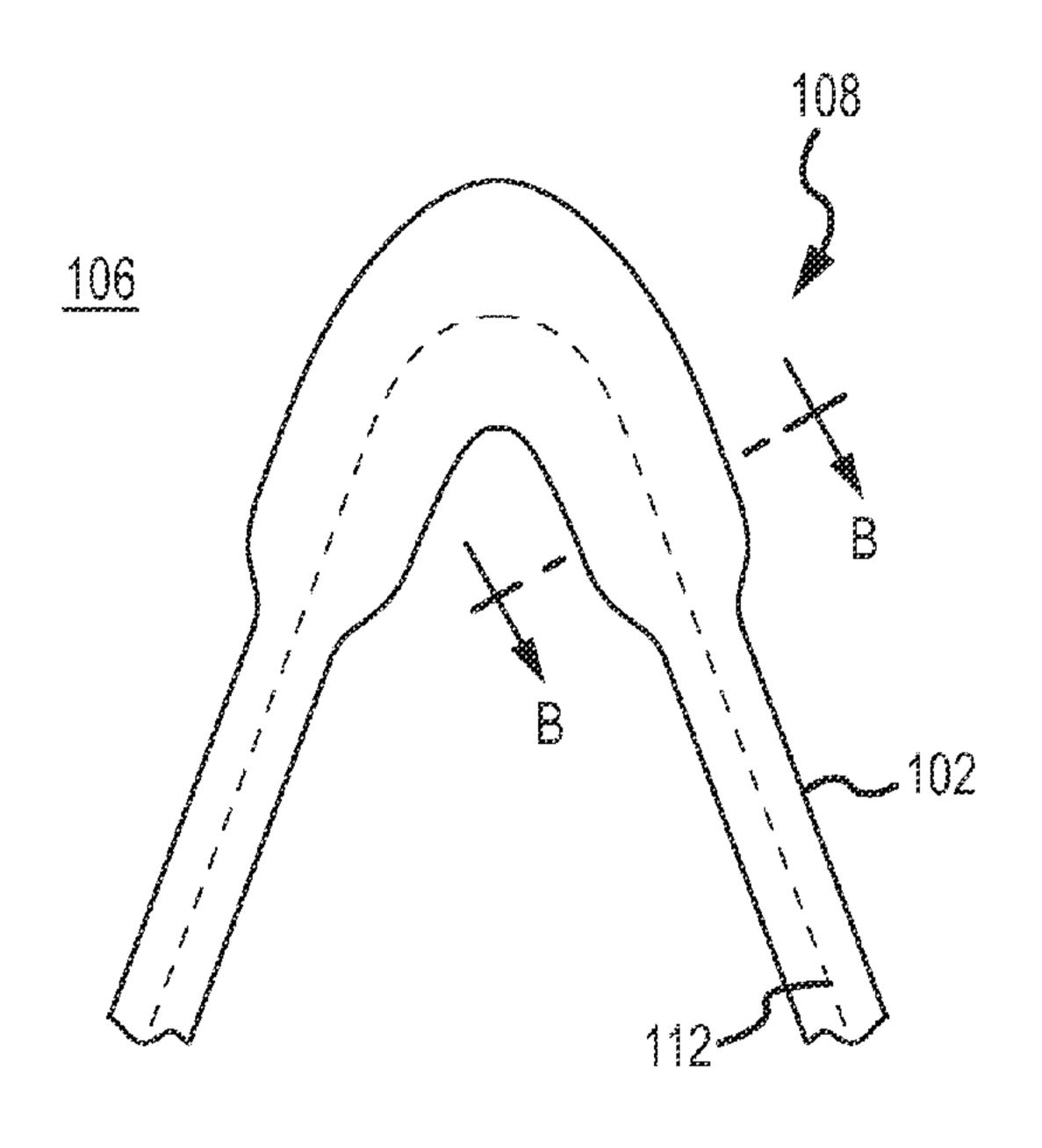
(57) Abstract: The present disclosure describes methods and apparatus for endoluminal devices, such as stents, that have components (102) with varying cross-sections (104) at various points about the length of the endoluminal device, with various benefits resulting therefrom.
