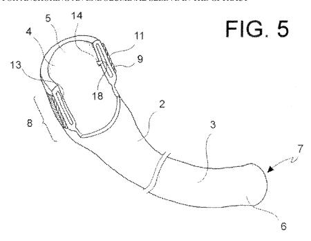
(57) Abstract: An endoluminal sleeve (2) for internally lining a section of a GI tract comprises a wall of a flexible material defining a sleeve lumen (3), a proximal end (4) defining a proximal lumen opening (5), a distal end (6) defining a distal lumen opening (7), and a tubular anchoring collar (8) formed at the proximal sleeve end (4) and having an external anchoring surface (9) with an adhesive layer (11).
