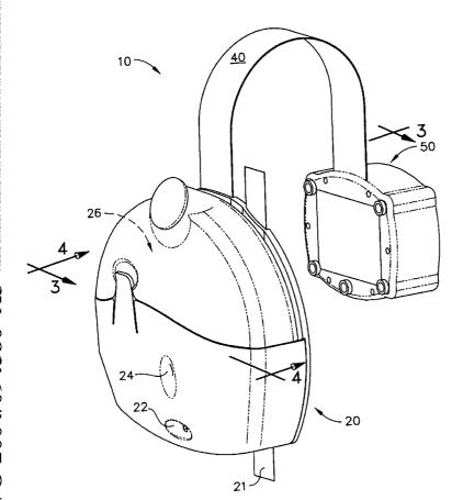
(57) Abstract: The present invention relates to methods of delivering one or more volatile materials, during the operation of a drying apparatus, to a fabric article. The present invention also relates to fabric treatment compositions comprising one or more volatile materials. These compositions may be used to treat fabric articles during the fabric article drying process.
