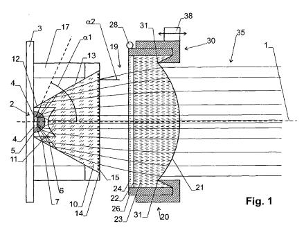
(57) Abstract: The illumination source has a LED light source (2) generating a first divergent light field (6). The light from the LED light source (2) is processed by a first optical element (10), in particular a first lens element, to generate a second divergent light field (19). The first divergent light field (19) is processed by a second optical element (20) having a variable lens variable focus in order to generate a third light field (35) whose divergence can be varied.
