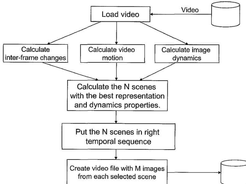
(57) **Abstract:** In a method for displaying video data within result presentations in information access or search systems, compressed thumbnails are computed for videos in a result page and applied to the result page. An end user is enabled to select a video in the result page and activate streaming of a video summary within the context of the associated result page.
