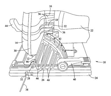
(57) Abstract: A circular saw has one or more louvers (36) in the housing which direct air exiting the housing toward a work piece, together with openings (46) in other components of the saw located between the louvers and the work piece so that sawdust and other debris that is produced during operation of the saw will be blown out of the way and will not interfere with the line of sight of the
