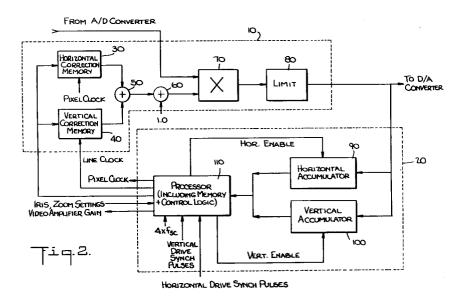
This invention relates to a method and apparatus for automatic white shading correction of video signals with the correction derived from using a flat white calibration target.
