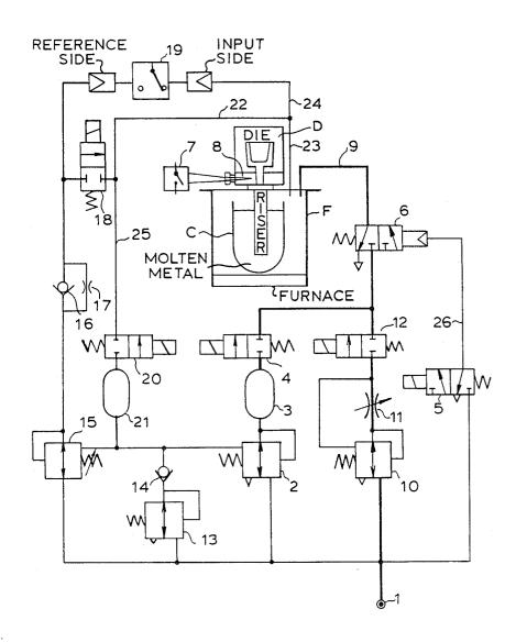
pressure in the furnace being maintained at a reference level of a value such that the difference between the after pressure and the datum pressure is maintained at a constant value despite changes in the level of molten metal in the furnace.
