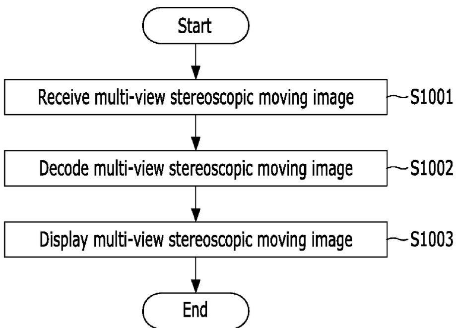
**APPARATUS AND METHOD FOR TRANSMITTING/RECEIVING MULTI-VIEW STEREOSCOPIC VIDEO**
