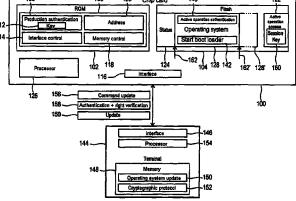
operating system and interrupting the execution of the chip card operating system following the start of the boot loader, reading the data from the predefined memory region by the boot loader, loading the program instructions from the chip card terminal into the NVM by the boot loader on the precondition that the data indicate the successful authentication and verification in the predefined memory region.
