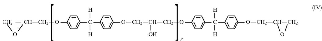
wherein  $p$  is usually an integer of from 0 to 33. BPFDEs useful in the present invention include mixtures of those of formula (IV) wherein values for  $p$  are different from each other. BPFDE preferably has a softening point of  $60^\circ$  to  $140^\circ$  C.
