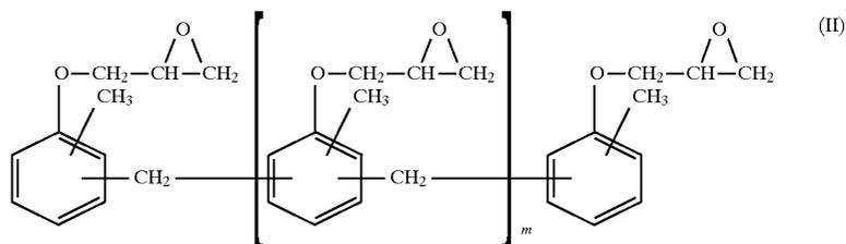
wherein m is usually an integer of from 3 to 7. CNPGEs useful in the present invention include mixtures of those of formula (II) wherein values for m are different from each other. CNPGE preferably has a softening point of 60° to 120° C.
