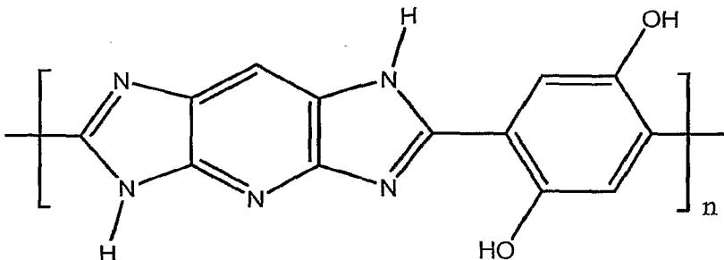
[0029] Polypyridobisimidazole fiber can be distinguished from the well known commercially available PBI fiber or polybenzimidazole fiber in that that polybenzimidazole fiber is a polybibenzimidazole. Polybibenzimidazole fiber is not a rigid rod polymer and has low fiber strength and low tensile modulus when compared to polypyridobisimidazoles.
