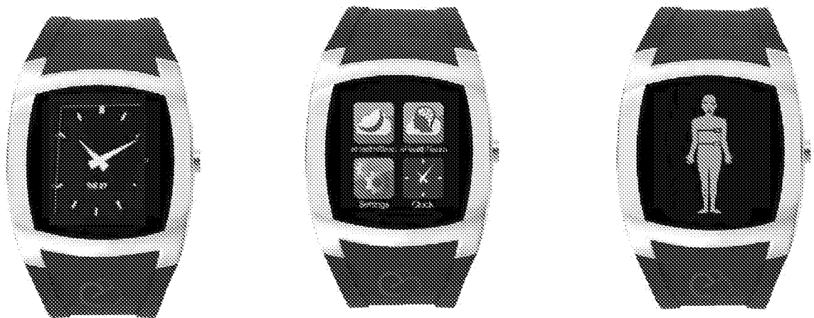
Figure 6 eHealthWATCH incorporating programmable watch face with health indications, health monitoring applications, monitoring setup and select applications, and sensor monitoring platform .
