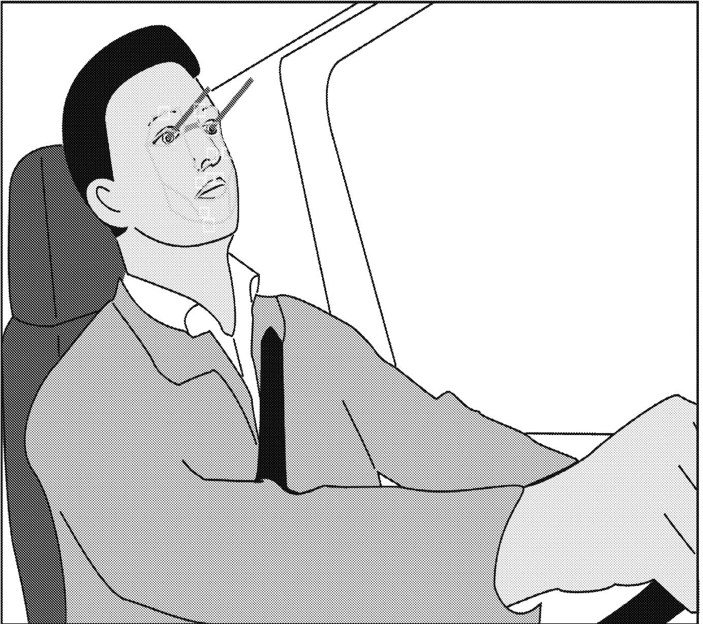
Figure 41 the present invention incorporates video imaging and associated facial feature recognition and tracking capabilities. >> the present invention enables monitoring and processing of driver/subject video in order to continuously determine head movements, drooping, rotation and other motion recognition and determination, along with associated facial feature recognition and associated motion changes, eye, gaze and other characteristics in order to detect changes applicable to driver drowsiness. Additionally, factors such as slowing eye-lid movements, extended driver/subject gaze or dwell and a decrease in normal vigilant behaviour can be continuously tracked as markers of driver drowsiness onset or changes in driver/subject attention or vigilance.
