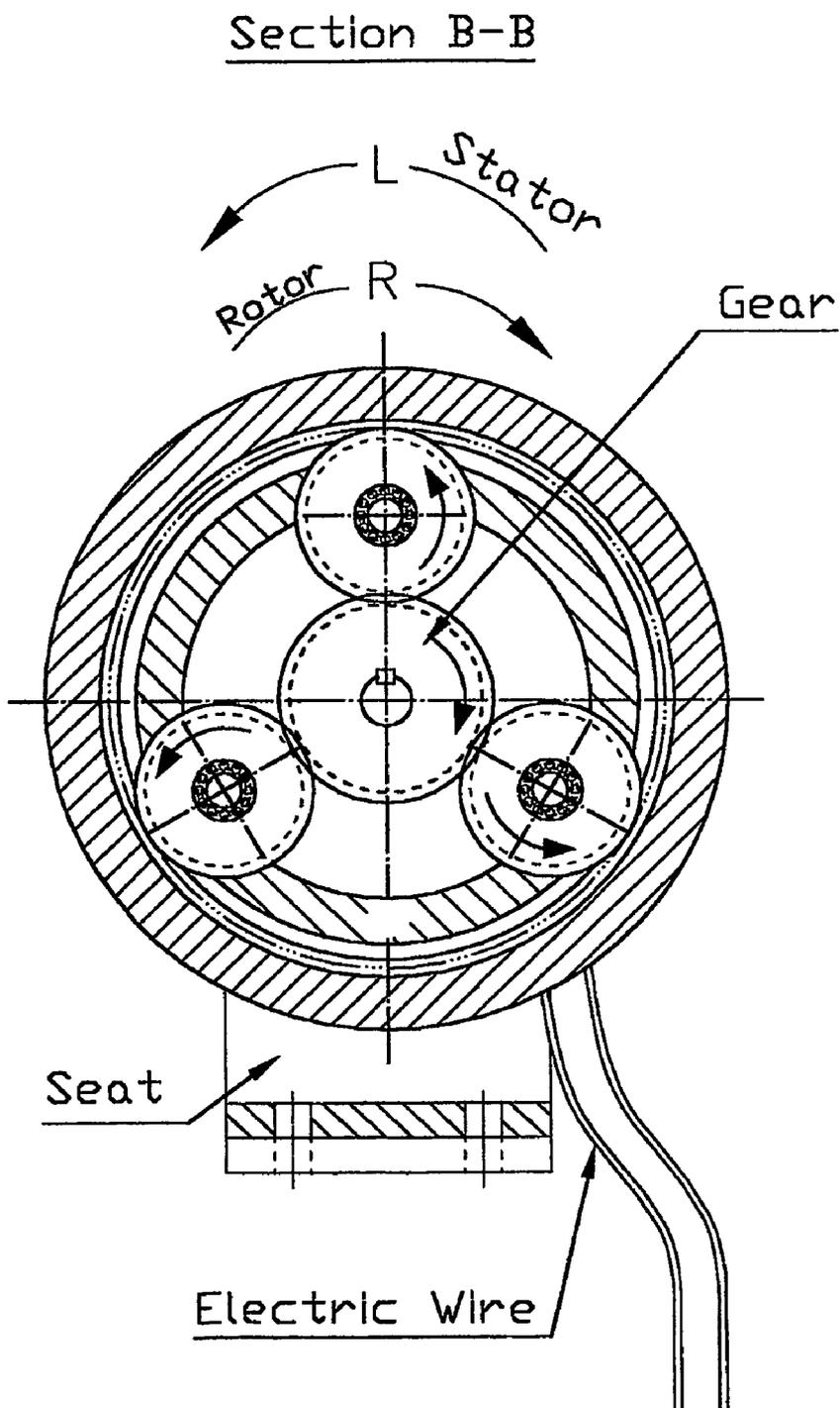
**MECHANISM FOR ROTATING THE ROTORS,
