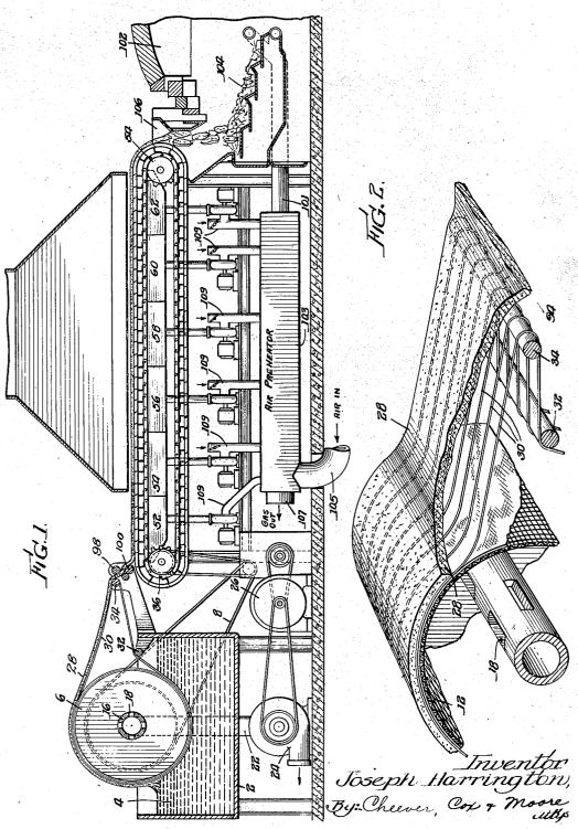
APPARATUS FOR DRYING AND DESTROYING SEWAGE
