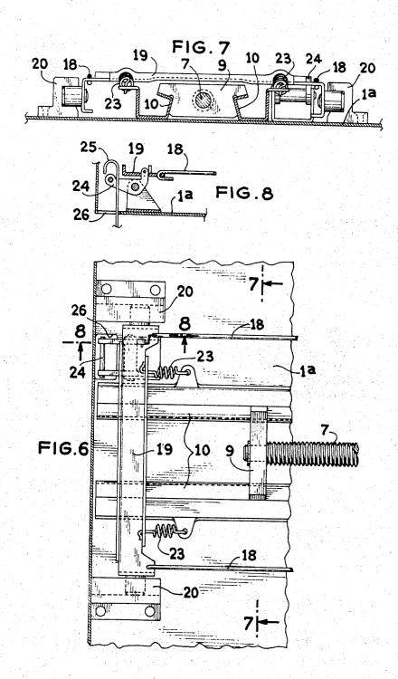
It is known that these sliding roofs can be actuated manually or electrically and that, in the first case, the moving panel is usually maintained in its partly opened position or fully opened position by the clamping of pads and the slideways which afford the lateral guides 10 for the panel. There is therefore a danger of an appreciable undesired sliding as a result of wear of the pads or insufficient clamping. Less frequently, the panel is held stationary by means of lateral locking mecha-
