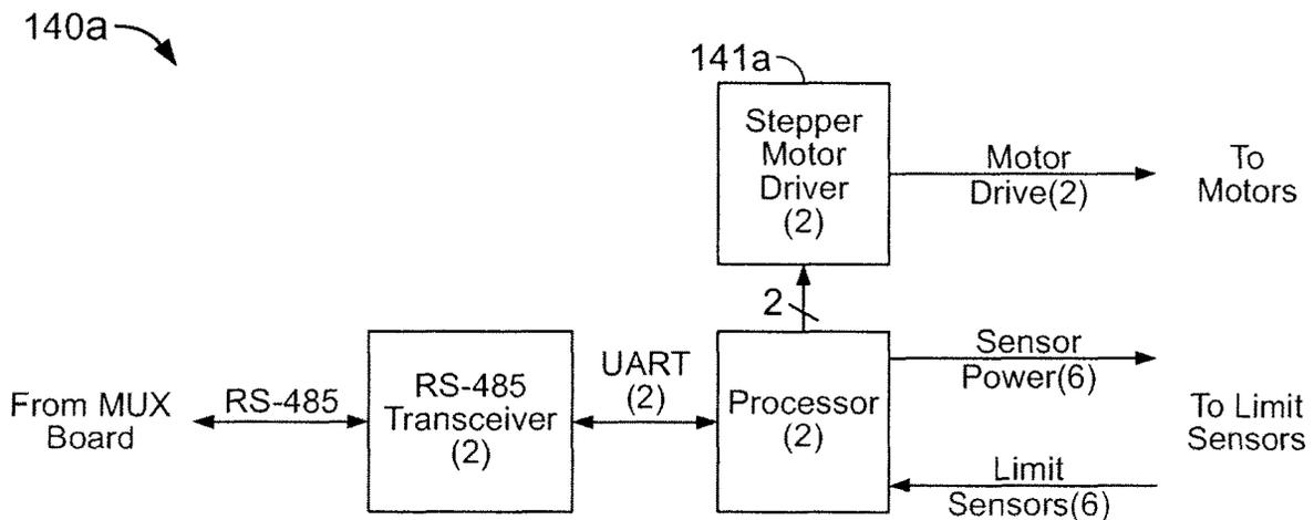
FIG. 91 Motor Control Board Block Diagram
