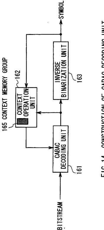
FIG. 14 CONSTRUCTION OF CABAC DECODING UNIT
