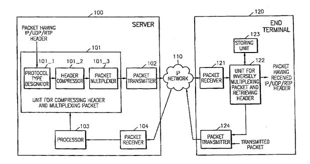
HAVING RECEIVED TERMINAL EN 9 TRANSMITTED PACKET UNIT FOR INVERSELY MULTIPLEXING PACKET AND RETRIEVING HEADER STORING RANSMITTER PACKET. RECEIVER PACKE NETWORK **FRANSMITTER** SERVER PACKET PACKET RECEIVER MULTIPLEXER PACKET 101\_3 UNIT FOR COMPRESSING HEADER AND MULTIPLEXING PACKET 100 101 PROCESSOR 101\_2 COMPRESSOR HEADER PROTOCOL TYPE DESIGNATOR 101
