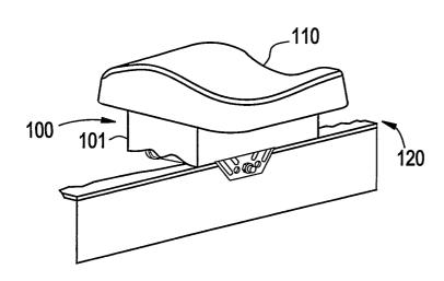
(57) Abstract: A stability adjustable unit for a seat of an exercise device that is configured for movement on the device may include a sub-assembly connected between the seat and a roller assembly of the device on which the The unit may include a seat rests. selector provided on the sub-assembly and operable by a user seated on the seat to vary a degree of stability of the seat.
