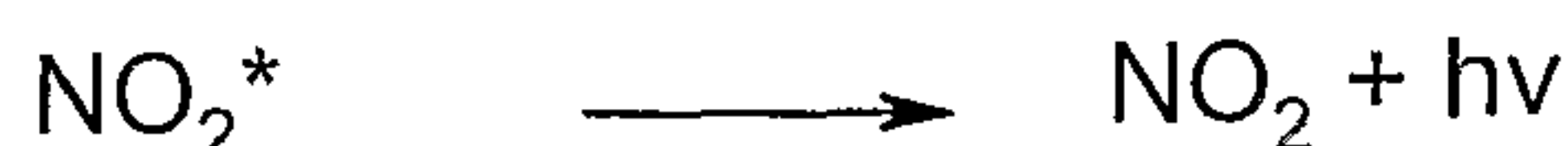
Scheme 2. Measurement of NO by chemiluminescence.
