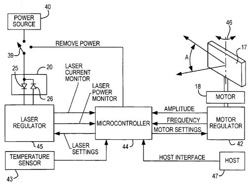
(57) Abstract: Laser power control arrangements interrupt power to a laser used in electro-optical readers upon detection of operating conditions not conforming to preestablished standards, and adjust power to the laser to enhance reader performance without violating prevalent safety standards.
