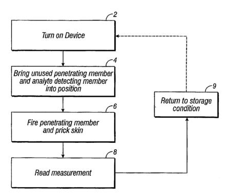
(57) Abstract: A method is provided for the analyte measurement by a user using an analyte measurement device. A penetrating member and unused analyte detecting member of the analyte measurement device are presented into an active position. The penetrating member is fired to prick the skin and bring a fluid sample to the analyte detecting member. The analyte level is measured. These three steps occur in less than 10 seconds.
