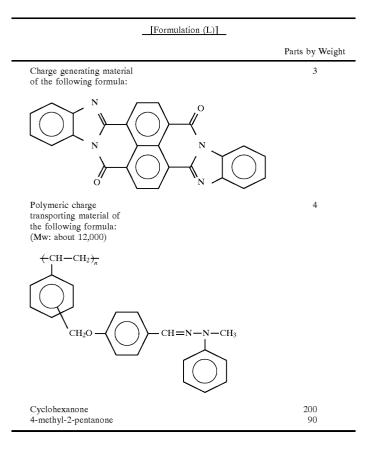
The thus prepared charge generation layer coating liquid was coated on the above prepared undercoat layer, and dried, so that a charge generation layer with a of 0.2  $\mu$ m was formed on the undercoat layer.
