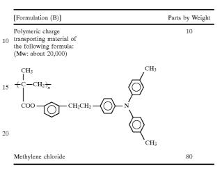
The thus prepared charge transport layer coating liquid was coated on the above prepared charge generation layer, and dried, so that a charge transport layer with a thickness of 24  $\mu$ m was formed on the charge generation layer.
