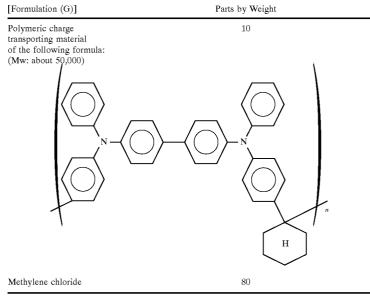
The thus prepared charge transport layer coating liquid was coated on the above prepared charge generation layer, 55 and dried, so that a charge transport layer with a thickness
