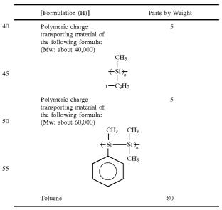
The thus prepared charge transport layer coating liquid was coated on an aluminum plate with a thickness of 0.2 mm serving as an electroconductive support, and dried, so that a charge transport layer with a thickness of  $20 \,\mu\text{m}$  was formed on the electroconductive support.
