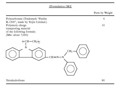
The thus prepared charge transport layer coating liquid wag coated on the above prepared charge generation layer, and dried, so that a charge transport layer with a thickness of 25  $\mu$ m was formed on the charge generation layer.
