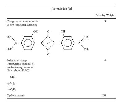
The thus prepared charge generation layer coating liquid was coated on the above prepared charge transport layer, and dried, so that a charge generation layer with a thickness of 0.4  $\mu$ m was formed on the charge transport layer.
