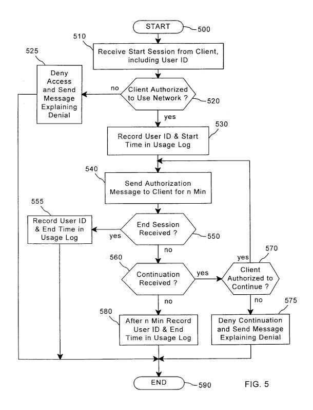
TWO-TIER AUTHENTICATION SYSTEM WHERE CLIENTS FIRST AUTHENTICATE WITH INDEPENDENT SERVICE PROVIDERS AND THEN AUTOMATICALLY **EXCHANGE MESSAGES WITH A CLIENT** CONTROLLER TO GAIN NETWORK **ACCESS**
