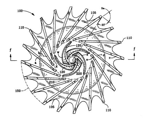
separate second plurality of vanes (120), by turning and pre-pressurizing the fluid, provides an impeller having capability of cavitation-free pumping at low net positive suction head (NPSH). A front shroud (180) can be used which partially or totally covers the first and/or second plurality of vanes.
