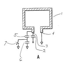
(57) Abstract: This invention relates to a method for improving the performance of a nuclear quadrupole resonance detection system by reducing the coupling between the excitation coil(s) that provide the radio frequency magnetic field that excites the quadrupole nuclei and the high temperature superconductor receive coil(s) that detect the resulting nuclear quadrupole resonance signal. The coupling is reduced by shifting the resonance frequency of the excitation coil(s) during signal reception.
