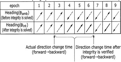
Latency occurs at the time of direction change but removal of distorted heading value is efficient
