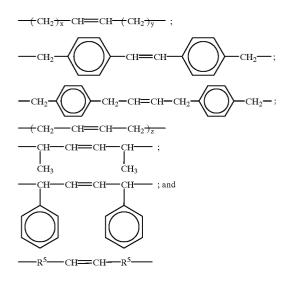
**[0034]** wherein x and y are individually selected from a group of integers of from 1 to 20 and the sum of x and y does not exceed 21; z is an integer of from 1 to 10; and  $R^5$  is a cycloaliphatic having from 5 to 8 carbon atoms in the ring. Preferably, x is from 2 to 4, y is from 2 to 4, z is 2 and R is a cycloaliphatic group having five carbon atoms in the ring. The siloxy compounds of Formula I may comprise a high purity product or mixture of products of the formula.
