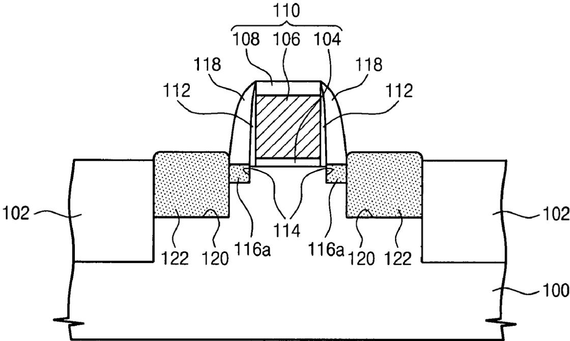
**SEMICONDUCTOR DEVICE INCLUDING FIELD EFFECT TRANSISTOR AND METHOD OF FORMING THE SAME**
