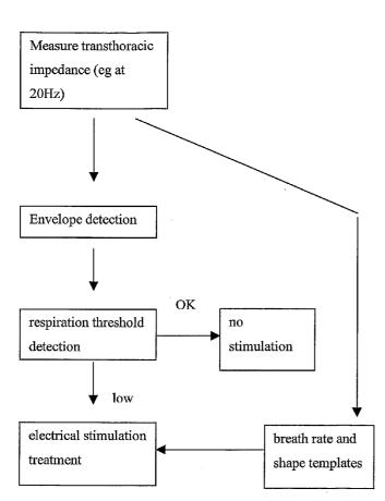
(57) Abstract: Methods and apparatus for detection and treatment of respiratory disorders using implanted devices are described. In one form, afferent nerves are electrically or electro-mechanically stimulated to increase the tone of upper airway muscles. Detection of respiratory disorders is carried out using electrodes implanted in sub-pectoral regions. Open and closed airway apneas are distinguished using a combination of acoustic detectors and electrical transducers.
